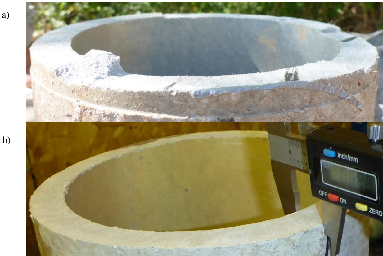
Figure 3-4. a) Surface before grinding; b) Measuring the pipe thickness after grinding
