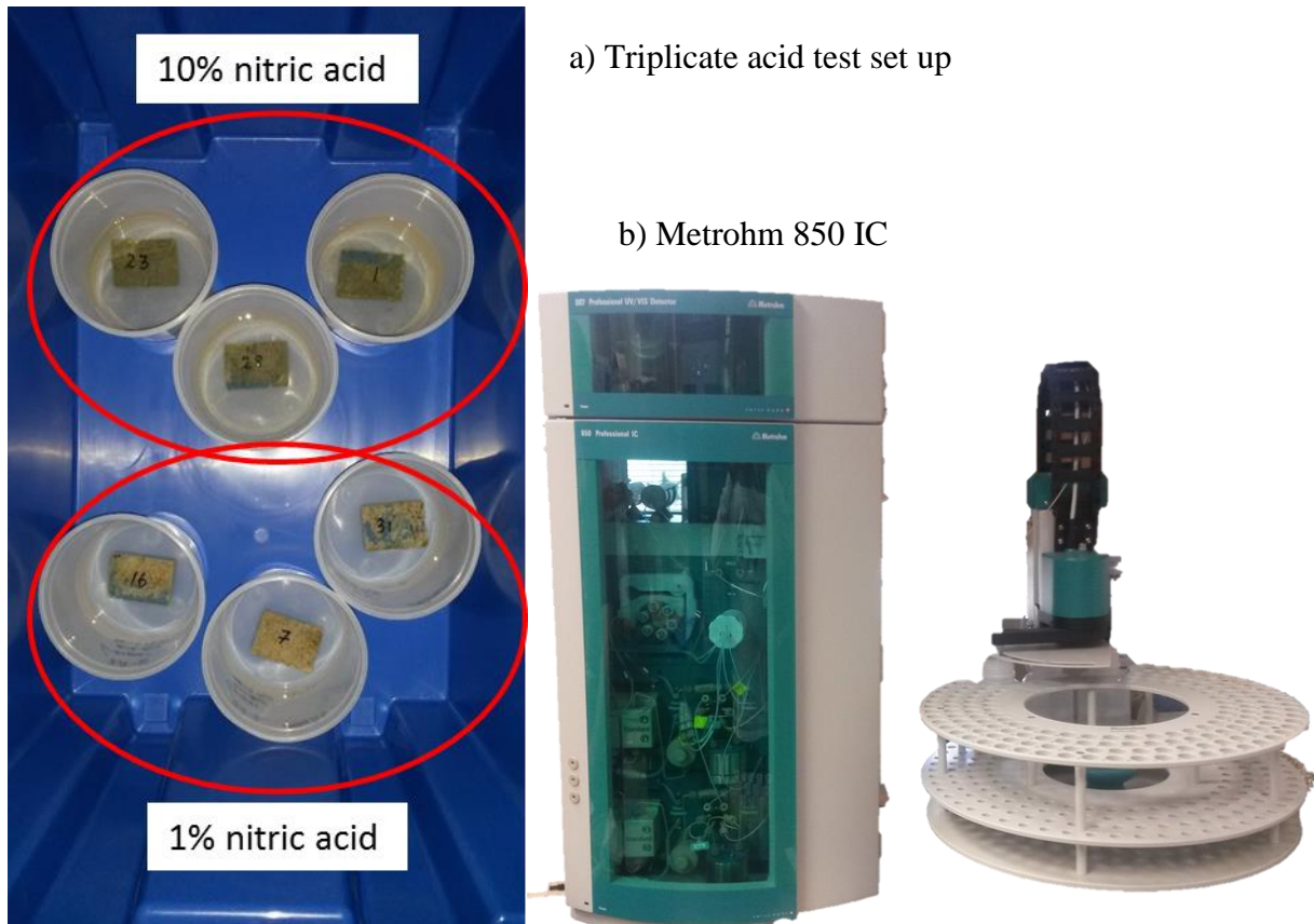
Figure 4-3. a) Sample set up for Phase II b) Ion Chromatograph
